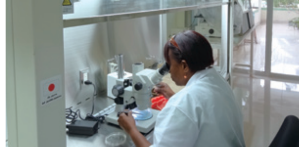
Clean benches and stereoscopic microscopes used for testing and research in aseptic conditions preventing the encroachment of bacteria (IDIAF)
