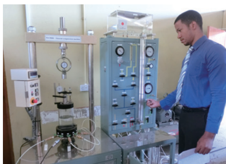
High-pressure triaxial compression machine procured for use in Grenada
