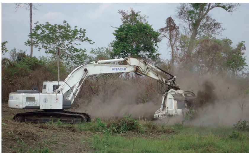
A landmine removal machine in action
