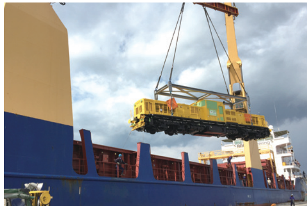
A diesel locomotive is lifted by crane onto the transport ship (Photo credit: Hokuriku Heavy Industries, Ltd.)
