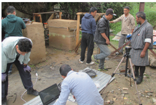
Testing the strength of test pieces used for traditional construction methods
