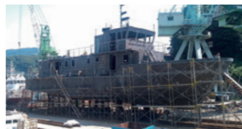
Medical ship for the Marshall Islands under ↑ construction on the slipway in June 2021 (Courtesy of Shipbuilding Research Centre of Japan)
