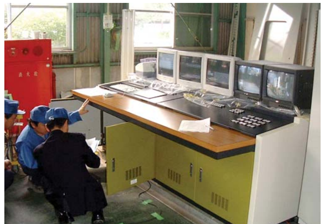
Support service for equipment procurement in Japan — JICS staff conducting pre-delivery check of centralized monitoring system for a coal mine
