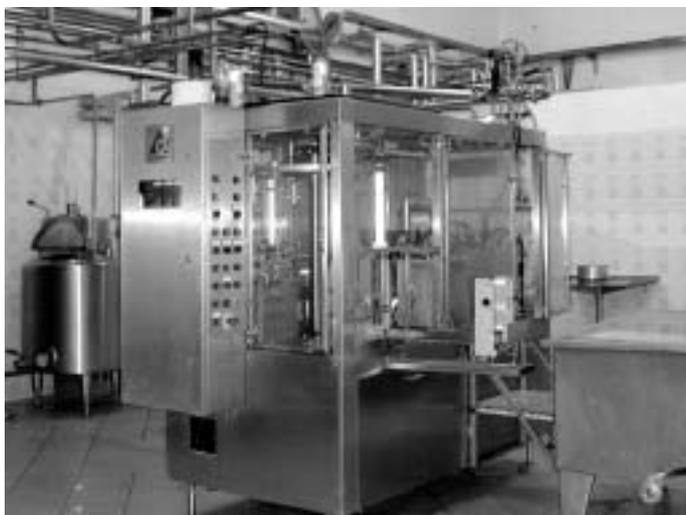
*Existing low-temperature milk sterilization equipment owned by a local milk processor.*
