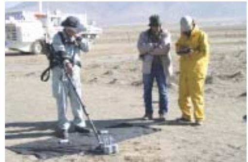
*Hand-held mine detector monitoring a buried dummy mine.*
