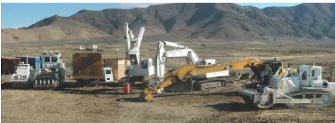
*The five types of demining equipment and a mine detector equipped vehicle that participated in testing.*
