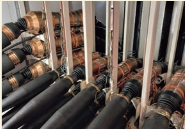
Optical submarine repeaters stored aboard a cable laying vessel
